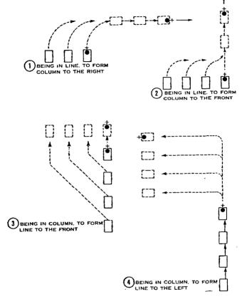
Figure 66. Moving vehicles changing direction of march in line or column.
